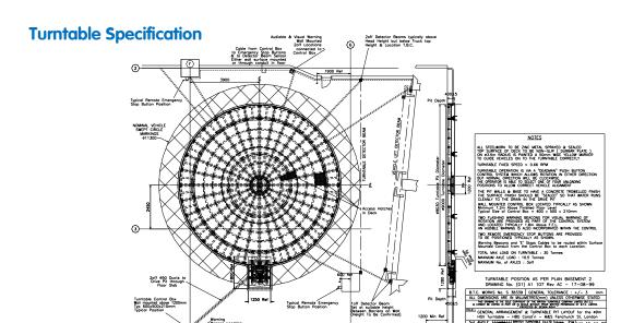
Construction: All steel construction, universal beam for main arms
